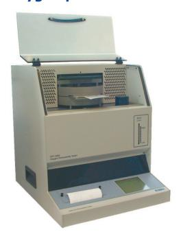
The OPT-5000 tester has been specifically developed to provide an easy and reliable test method. With a minimum of training anybody can perform a quality test. Just insert the sample, choose the test programme and press START - that's it! The user interface is based upon an easy to use touch screen display, which indicates the test cycle and the oxygen transmission rate as the testing progresses.
