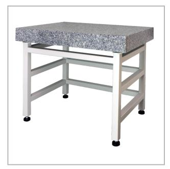
Labolatory table SAL/STONE is designed for ensuring stable operating conditions in high precision weighing applications. The table top is manufactured from polished granite based on mild steel, metal construction. Robust construction of the table along with special vibrationabsorbersensureexcellentisolationofmeasuringinstruments from possible vibrations, sourcing from environmental factors. Adjusting the level is possible with the use of adjusting feet mounted at the base of the table.
